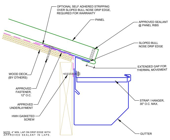
NOTE: PERIMETER CLEAT FASTENED WITH 12 GA. ANNULAR RING SHANK NAIL OR #10 DIAMETER SCREW, 10" O.C.AT PERIMETER ROOF AREAS AND 6" O.C. AT CORNER ROOF AREAS.
