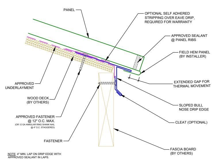
NOTE: PERIMETER CLEAT FASTENED WITH 12 GA. ANNULAR RING SHANK NAIL OR #10 DIAMETER SCREW, 10" O.C.AT PERIMETER ROOF AREAS AND 6" O.C. AT CORNER ROOF AREAS.
