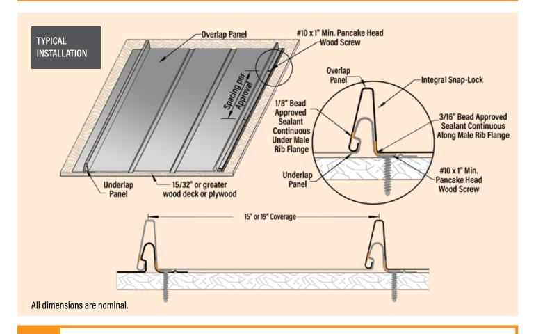
Actual fastener pattern may vary from the pattern shown based on the specific roof plan, metal type and strength, local building codes and product approvals.
