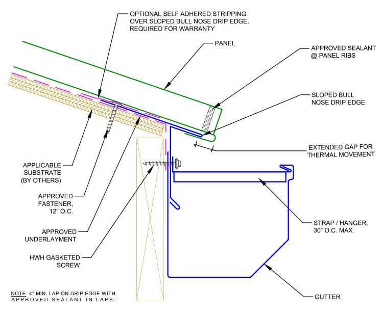
$\underline{\text{NOTE}}:$  PERIMETER CLEAT FASTENED WITH 12 GA. ANNULAR RING SHANK NAIL OR #10 DIAMETER SCREW, 10" O.C.AT PERIMETER ROOF AREAS AND 6" O.C. AT CORNER ROOF AREAS.
