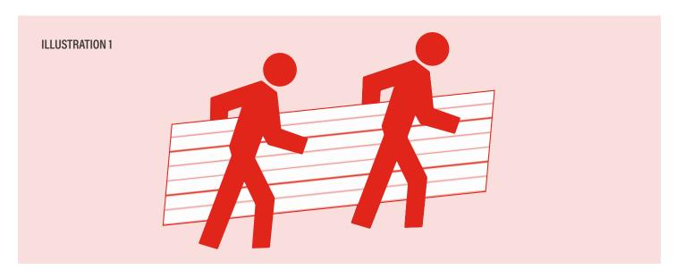
Once a bundle is opened, individual panels must be handled with care to prevent panel buckling or finish damage. Never slide a panel over another panel when removing it from the bundle. A panel should be lifted up from the bundle in order to minimize the possibility of damaging the finish.
