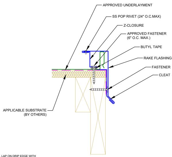
$\underline{\mathsf{NOTE}} : \mathsf{4"}$  MIN. LAP ON DRIP EDGE WITH APPROVED SEALANT IN LAPS.
