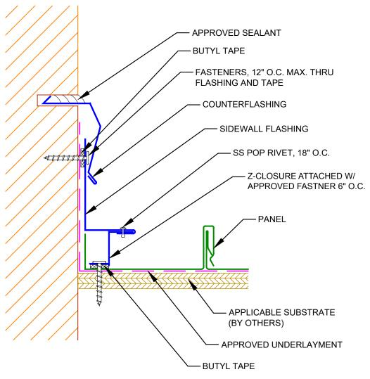
$\underline{\text{NOTE}};$  6" MIN. LAP ON SIDEWALL FLASHING WITH APPROVED SEALANT IN LAPS.
