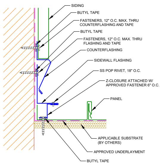
$\underline{\text{NOTE}}\textsc{:}$  6" MIN. LAP ON SIDEWALL FLASHING WITH APPROVED SEALANT IN LAPS.
