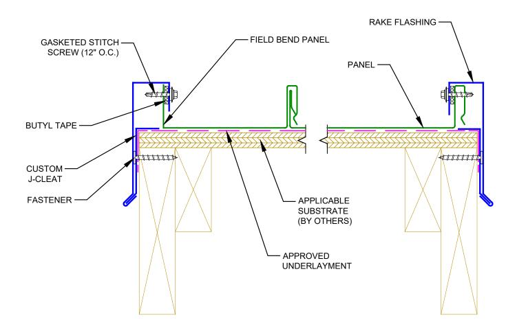
$\underline{\text{NOTE}}\textsc{:}$  4" MIN. LAP ON RAKE DRIP EDGE WITH APPROVED SEALANT IN LAPS.
